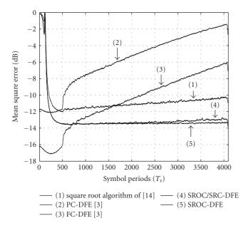
FIGURE 4: Convergence and tracking performance of equalizers for a  $4 \times 4$  system trained for  $512T_s$ , and operating over a time-varying, frequency-selective MIMO channel at SNR = 16 dB. The normalized Doppler frequency is  $5.5 \cdot 10^{-5}$ .
