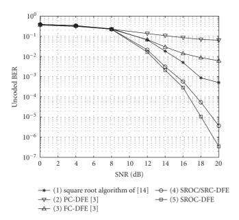
FIGURE 5: Uncoded BER curves of equalizers for a  $4 \times 4$  system trained for  $512T_s$ , and operating over a time-varying frequency-selective MIMO channel with a normalized Doppler frequency of  $5.5 \cdot 10^{-5}$ .
