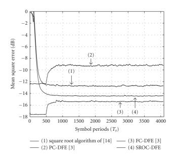
FIGURE 3: Convergence and steady-state performance of equalizers for a  $4 \times 4$  system trained for  $512T_s$ , and operating over a static frequency-selective MIMO channel at SNR = 16 dB.
