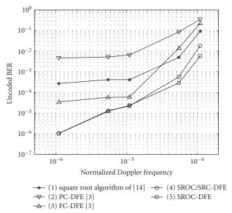
FIGURE 6: Uncoded BER of equalizers for a  $4 \times 4$  system trained for  $512T_s$ , and operating over a time-varying frequency-selective MIMO channel at SNR =  $16 \, \text{dB}$ . The normalized Doppler frequency ranges from  $1 \cdot 10^{-6}$  to  $1 \cdot 10^{-4}$ .
