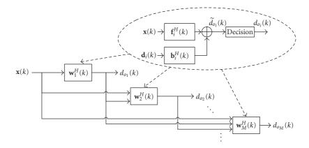
FIGURE 1: Adaptive BLAST MIMO decision feedback equalizer architecture.
