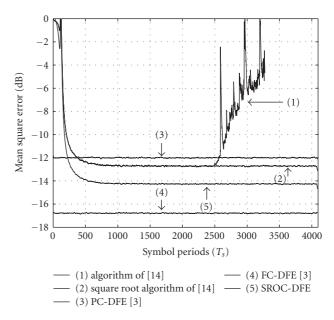
FIGURE 2: Convergence and steady-state performance of equalizers for a  $4 \times 4$  system operating constantly in training mode over a static frequency-selective MIMO channel at SNR = 16 dB.
