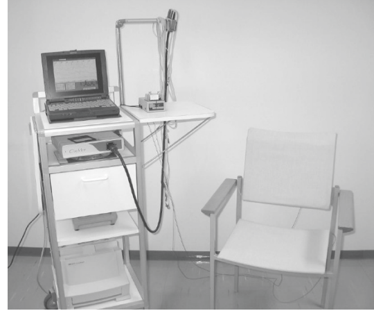
FIGURE 2: A chair equipped with an EMFi-film sensor, the charge amplifier, a CircMon device, and a laptop PC.
