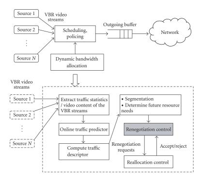
FIGURE 1: Dynamic bandwidth allocation architecture.
