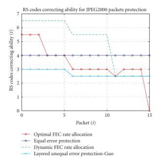
FIGURE 12: Correcting ability of the RS(n,32) codes used for JPEG 2000 data packets—bandwidth of 6 Mbps.
