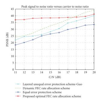
FIGURE 14: PSNR versus carrier-to-noise ratio.
