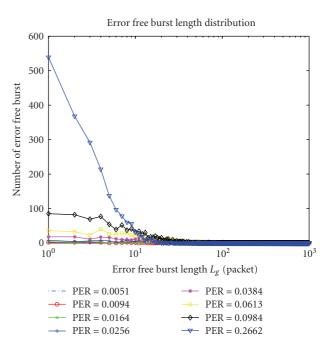
FIGURE 7: Error-free burst length distribution.
