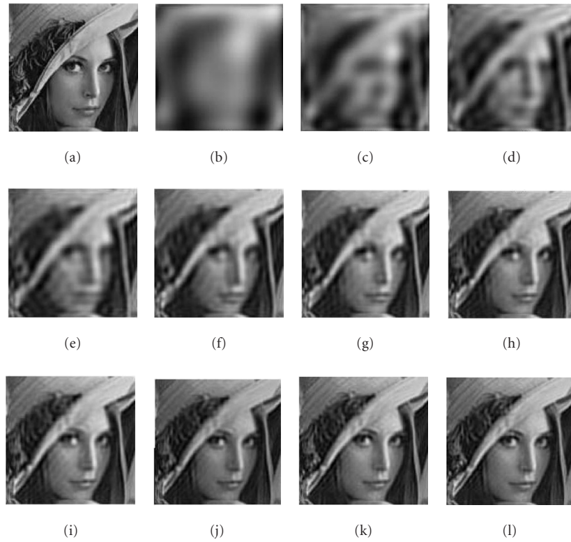
FIGURE 9: Global reconstruction of the Lena image by the Legendre moments. (a) Original input image; reconstructed images from (b) to (l) represent orders 10, 20, 30, 40, 50, 60, 70, 80, 90, 100, and 110, respectively.
