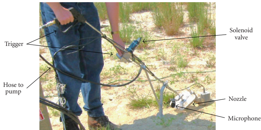
FIGURE 7: The waterjet lance used to collect data in the field.
