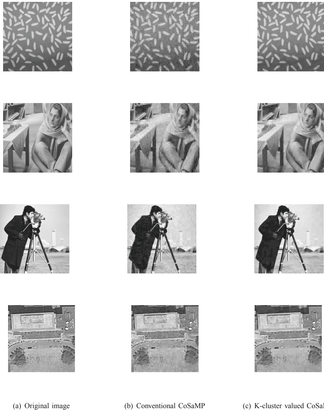
Figure 7 (a) The original gray images measured by CS with wavelet sparsity basis. The measurement numbers of both conventional and K -cluster-valued CS over these images are M = 3.5S , where S is the number of compressible wavelet coefficients greater than threshold 20. (b) The reconstructed images using the conventional CoSaMP recovery method. (c) The images reconstructed by K -cluster-valued (wavelet coefficients) CoSaMP. Note that cluster number K was chosen to be 40 for all these images.
