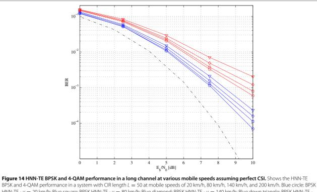
BPSK and 4-QAM performance in a system with CIR length L = 50 at mobile speeds of 20 km/h, 80 km/h, 140 km/h, and 200 km/h. Blue circle: BPSK HNN-TE - v = 20 km/h; Blue square: BPSK HNN-TE - v = 80 km/h; Blue diamond: BPSK HNN-TE - v = 140 km/h; Blue down triangle: BPSK HNN-TE v = 200 km/h; Red circle: 4-QAM HNN-TE - v = 20 km/h; Red square: 4-QAM HNN-TE - v = 80 km/h; Red diamond: 4-QAM HNN-TE - v = 140 km/h; Red down triangle: 4-QAM HNN-TE - v = 200 km/h; Black dashed: coded AWGN bound.
