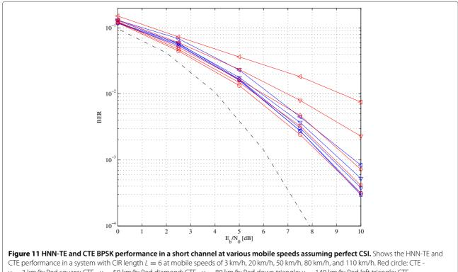
v = 3 km/h; Red square: CTE - v = 50 km/h; Red diamond: CTE - v = 80 km/h; Red down triangle: v = 140 km/h; Red left triangle: CTE - v = 200 km/h; Blue circle: HNN-TE - v = 3 km/h; Blue square: HNN-TE - v = 50 km/h; Blue diamond: HNN-TE - v = 80 km/h; Blue down triangle: HNN-TE - v = 140 km/h; Blue left triangle: HNN-TE - v = 200 km/h; Black dashed: coded AWGN bound.
