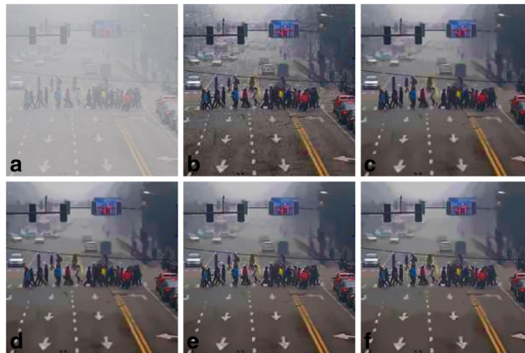
Figure 5 The third real data set. (a) The original true degraded data. (b) DC. (c) IR with denoising in the first stage. (d) DC-NL with denoising in the first stage. (e) IR with deblurring and denoising in the first stage. (f) DC-NL with deblurring and denoising in the first stage.
