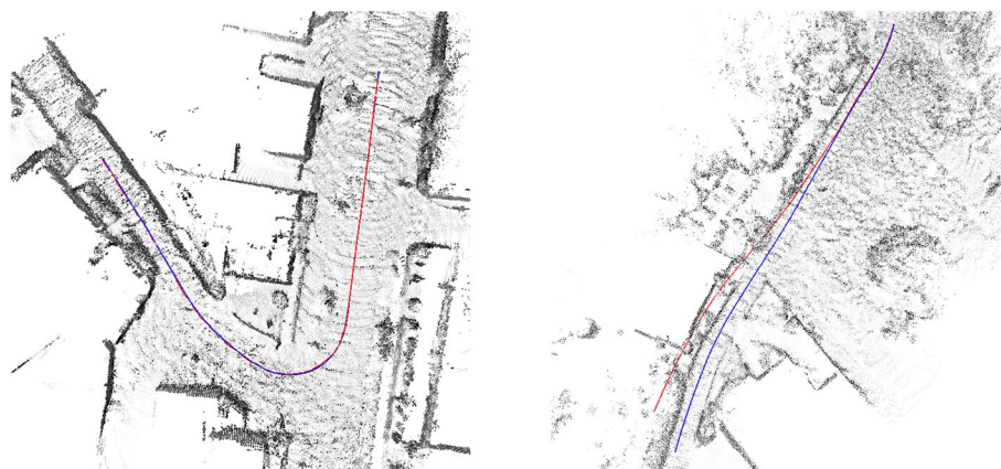
Fig. 12 Outdoor navigation example using the proposed PCMN on the KITTI dataset. Ground truth trajectory is shown in blue, and estimated trajectory is shown in red. Initialization was identical in all examples (see Sect. 4.2). Left: Drift-free map-based tracking using the 3DMMD. Right: Accumulated drift using differential tracking
