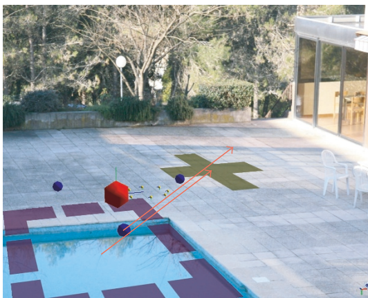
FIGURE 16: An example interface for source relocalization. In this example, we select the area corresponding to the fountain (in purple) and translate it to a new location (shown as a yellow cross). The listener is depicted as a large red sphere, the microphone array as small yellow spheres, and the blue spheres show cluster locations.
