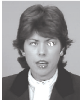
FIGURE 7: Image from visual telephone image sequence “Claire” with detected eye regions marked in black or white.
