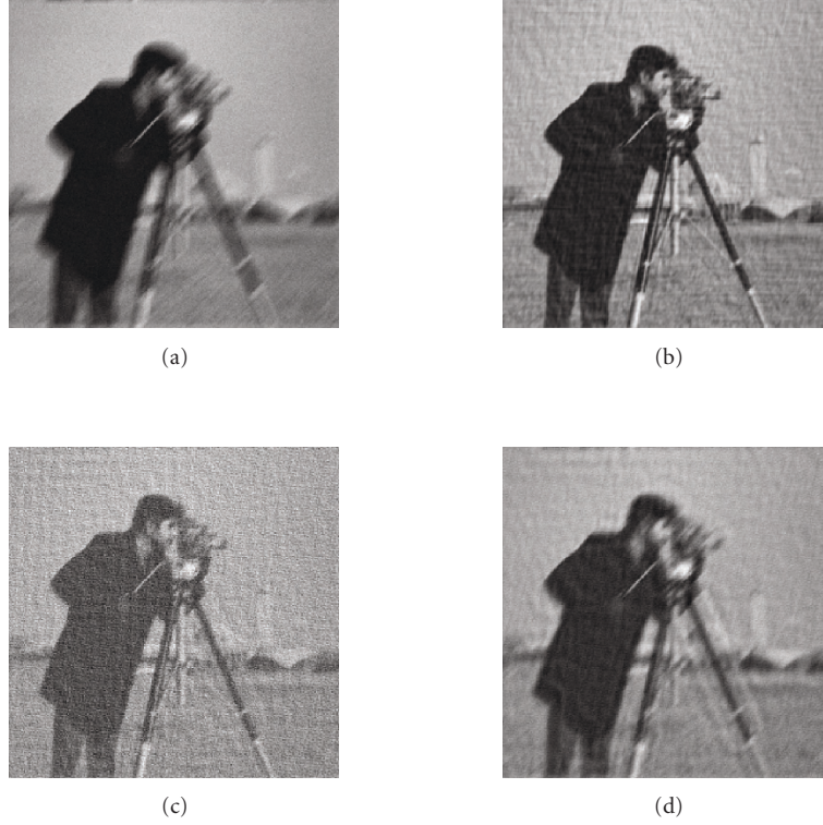
FIGURE 7: From Figure 6, we take a specific pair of values (\text{BSNR}, \varepsilon_\sigma) = (20 \text{ dB}, 80\%) showing the degraded image \mathbf{y} in (a) and the restored images \hat{\mathbf{x}} in (b), (c), and (d) when, respectively, obtained by the Wiener filter with optimum estimates ( \text{ISNR} = 4.14 \text{ dB} ), the same when an error of \varepsilon_\sigma is applied on the noise variance ( \text{ISNR} = -3.25 \text{ dB} ) and the last one when our proposed desensitisation method is used with the same error ( \text{ISNR} = 1.44 \text{ dB} ).
