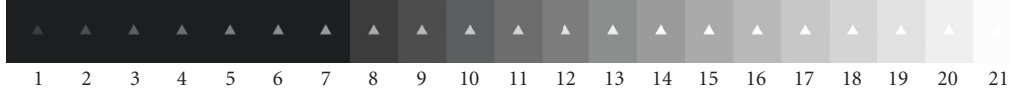
FIGURE 1: Example of a test image of triangles with changed brightness. The original image is the 7th image.
