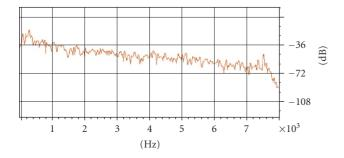
FIGURE 6: Long-term power spectrum of office noise used in the experiments.
