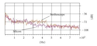
FIGURE 7: Long-term power spectrum of office noise at 70 dBA level captured by NAM microphones.
