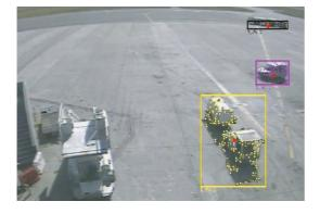
FIGURE 9: Detected object locations (red circles) shown for 3 vehicles in the near-, mid-, and far-field of Camera 5 for sequence S4.
