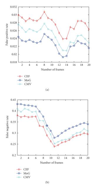
FIGURE 12: (a) false positive and (b) false negative error rates versus number of frames for Dataset S21.
