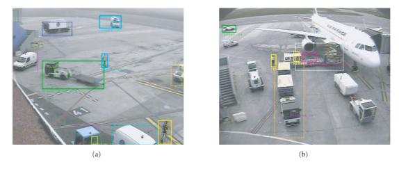
FIGURE 14: The results obtained from the local feature-based tracking algorithm. Image (a) has been chosen from S21-Cam7 and image (b) from S28-Cam5.
