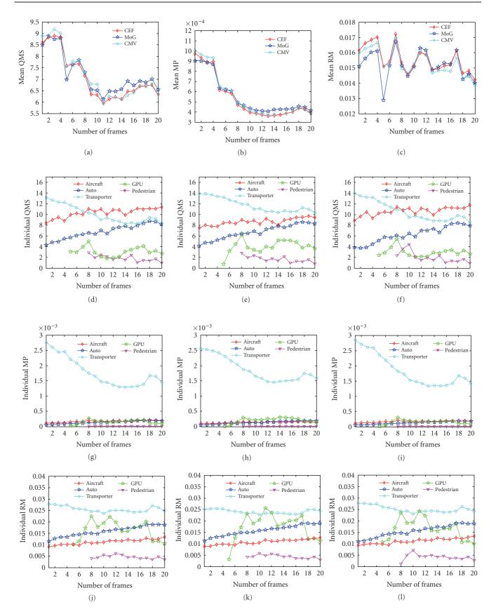
FIGURE 13: Average and individual object segmentation errors for Dataset S21; (a), (b), (c) average QMS, MP, and RM object-based segmentation errors of the motion detectors; (d), (e), (f) QMS individual object segmentation error of CEF, MoG, and CMV; (g), (h), (i) MP individual object segmentation error of CEF, MoG, and CMV; (j), (k), (l) RM individual object segmentation error of CEF, MoG, and CMV.
