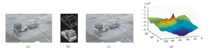
FIGURE 8: (a) Frame of sequence S21 showing a transporter vehicle. (b) Edge-based and appearance-based 3D model for the transporter vehicle. (c) The appearance model fitted to the vehicle, with the ground-plane (x, y) search area shown in blue. (d) x-, y-slice of the evaluation score surface in the (x, y,  $\theta$ ) search space.
