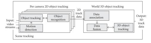
FIGURE 3: The scene tracking module in the AVITRACK system.
