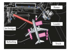
FIGURE 1: The distribution of equipment around an A320 aircraft on apron echo-40 at Toulouse Airport, France.
