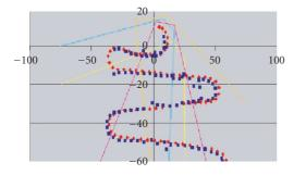
FIGURE 17: Vehicle 2D trajectory graph showing (red) the EGNOS trajectory and (blue) the estimated location on the apron. The scale is measured in metres and the camera fields of view are shown.
