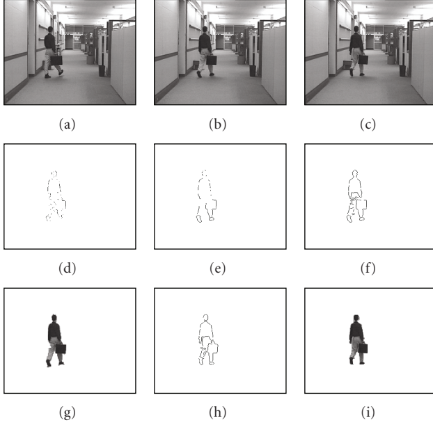
FIGURE 8: Detection and segmentation of moving object in “Hall Monitor” sequence. (a) I_{46} ; (b) I_{47} ; (c) I_{48} ; (d) detected moving edges of I_{47} by DC ; (e) detected moving edges of I_{47} by SD ; (f) detected moving edges of I_{47} by the proposed method; (g) segmented moving edges by of I_{47} the proposed method; (h) moving edges of I_{48} by the proposed method; (i) segmented moving object of I_{48} by the proposed method.
