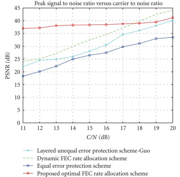
FIGURE 14: PSNR versus carrier-to-noise ratio.
