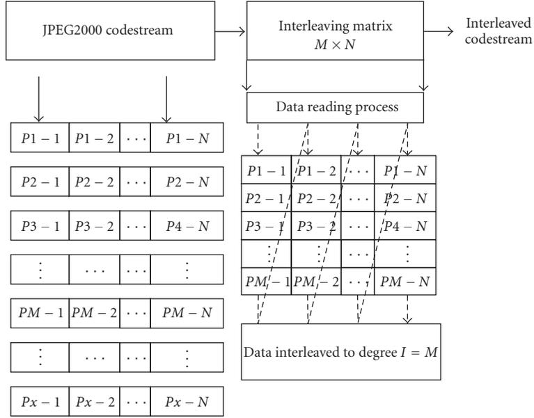
FIGURE 10: Interleaving process.
