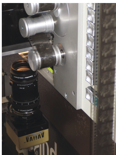
FIGURE 5: Close shot of our specific scanner, showing the line-scan camera and macro lens.
