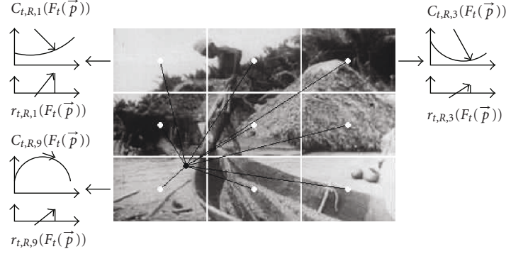
FIGURE 7: Block-based partition of the first frame of Boat using a 3 \times 3 grid. The pixel undergoing compensation and the centre of each block are represented by black and white dots, respectively. The black lines represent the Euclidean distances c_b(p) . Polynomial correction profiles C_{t,ref,b} and associated reliabilities r_{t,ref,b} are available for each block b . Compensation value for pixel \vec{p} is obtained by a bilinear interpolation of the block-based compensation values (9 in this example). Bilinear interpolation involves weighting by block-based reliabilities and distances d_b .
