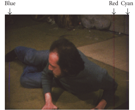
FIGURE 2: Degraded frame with three common types of scratch. From left to right: blue, red, and cyan.
