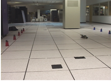
FIGURE 9: Picture of the testbed. Sensors can be seen on the left, lasers on the right. The car that was used as an “object” can be seen in the middle.
