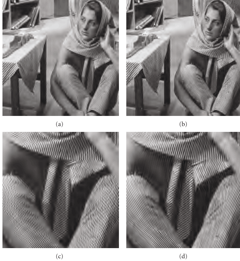
FIGURE 21: Reconstructed Barbara images at 0.15 bpp using (a) JPEG2000, PSNR = 25.93 dB and (b) PDFB, PSNR = 26.74 dB. (c) and (d) are zoom-in images of (a) and (b), respectively.
