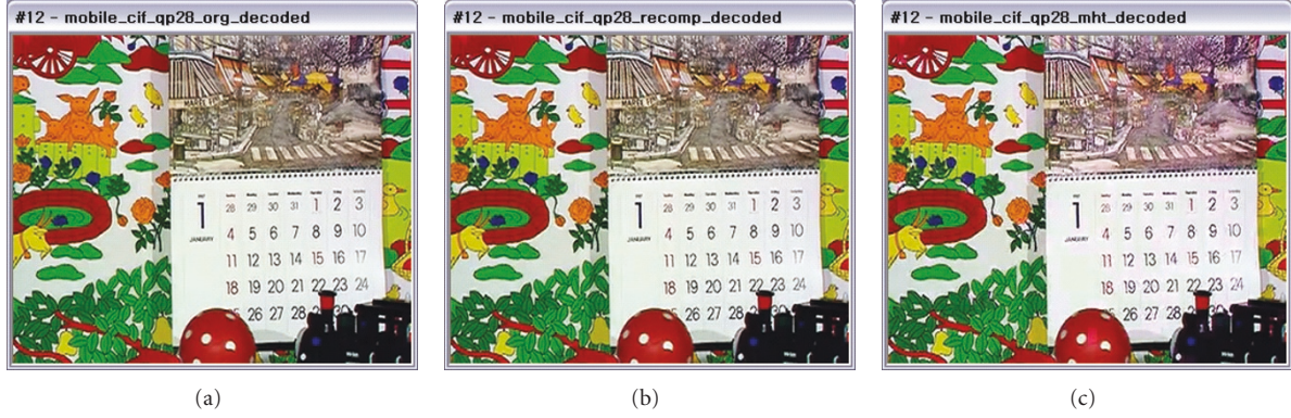
FIGURE 13: Subjective quality comparison for Mobile Calendar sequence: (a) original H.264, (b) H.264 + Proposed FMC, and (c) H.264 + MHT-based FMC.
