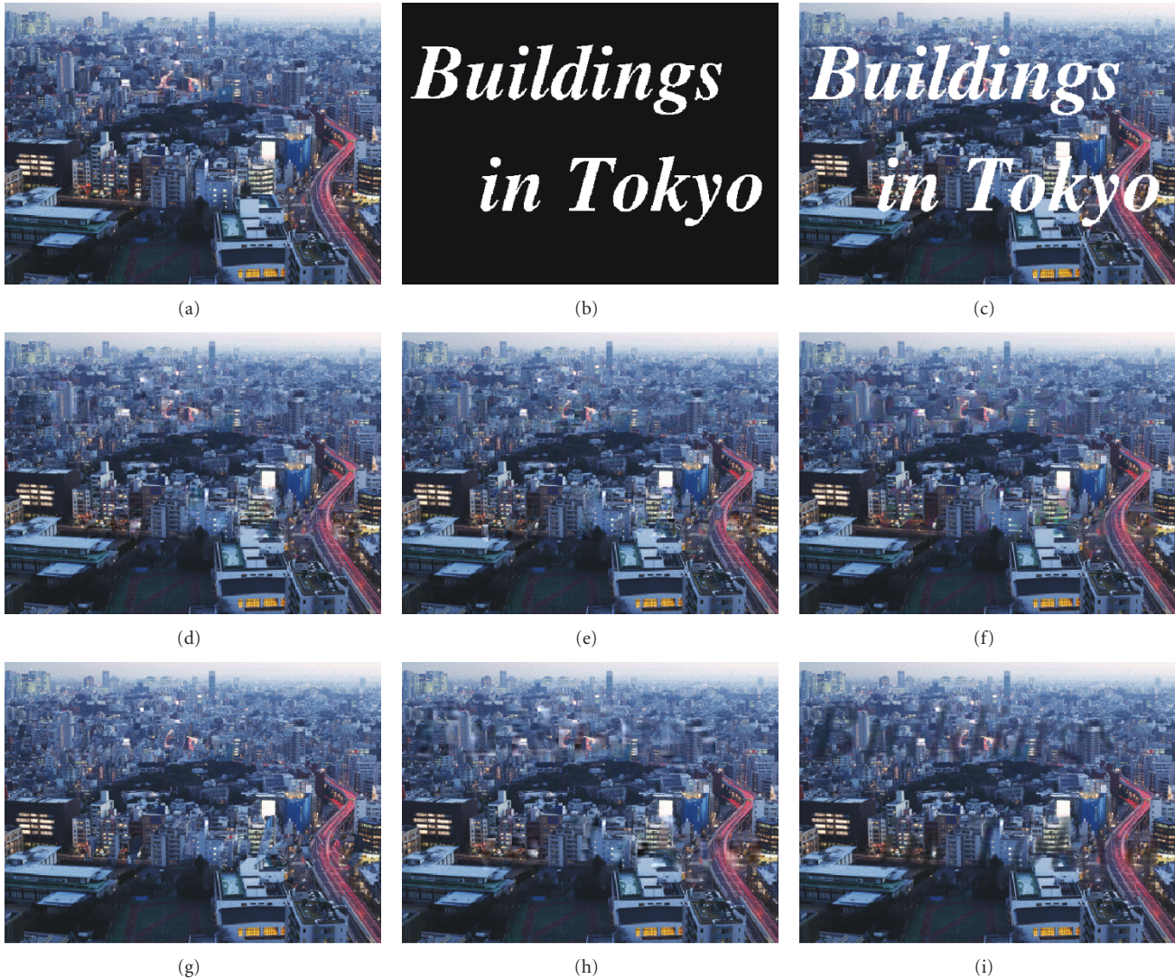
FIGURE 4: (a) Original image ( 480 \times 360 pixels, 24-bit color levels). (b) Flag image whose white regions correspond to missing areas. (c) Corrupted image including text regions (10.7% loss). (d) Reconstructed image by the proposed method. (e) Reconstructed image by the method based on the random selection. (f) Reconstructed image by the method which utilizes the MSE instead of the SSIM index. (g) Reconstructed image by the conventional method [11]. (h) Reconstructed image by the conventional method [13]. (i) Reconstructed image by the conventional method [21].
