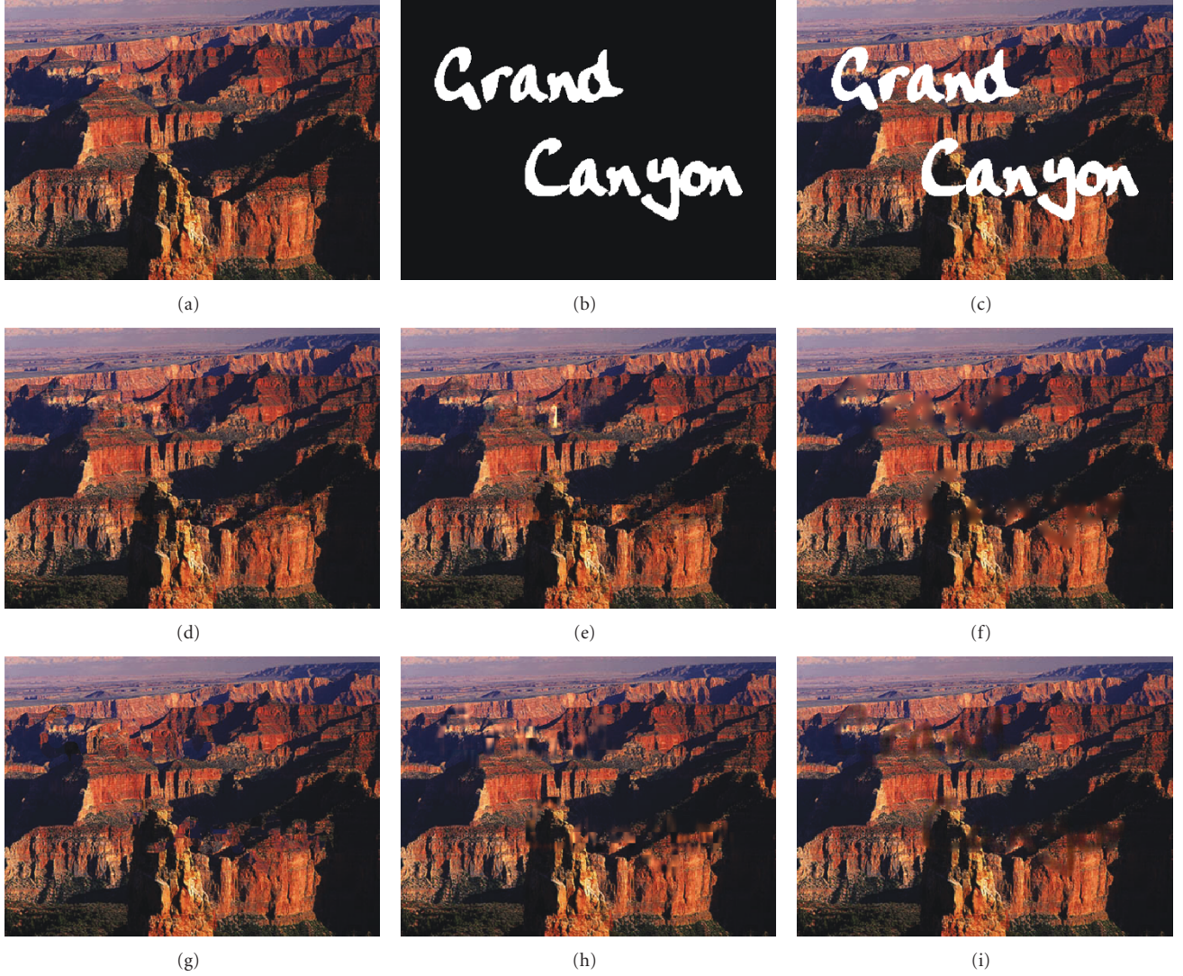
FIGURE 2: (a) Original image ( 480 \times 359 pixels, 24-bit color levels). (b) Flag image whose white regions correspond to missing areas. (c) Corrupted image including text regions (8.9% loss), (d) Reconstructed image by the proposed method. (e) Reconstructed image by the method based on the random selection. (f) Reconstructed image by the method which utilizes the MSE instead of the SSIM index. (g) Reconstructed image by the conventional method [11]. (h) Reconstructed image by the conventional method [13]. (i) Reconstructed image by the conventional method [21].
