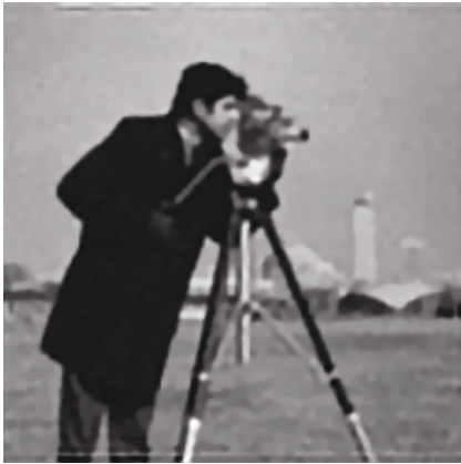
FIGURE 10: Artifacts appeared when removing the boundary conditions, cropping the center, in a MM1 algorithm. With zeros outside, the restoration is completely corrupted.
