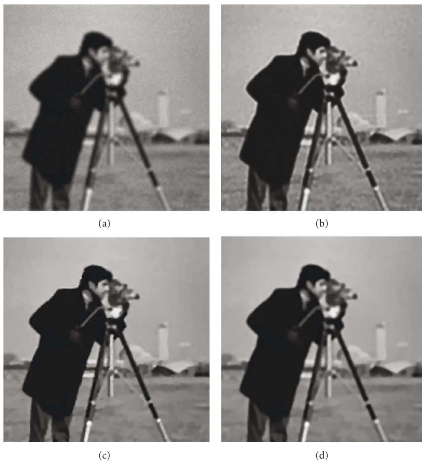
FIGURE 11: Restoration results from the Cameraman degraded image by Gaussian blur 7 \times 7 , BSNR = 20 dB and CIR model (a). The restored images are shown for (b) \ell_1 -MLP: \sigma_e = 15.55 , (c) MM2: \sigma_e = 14.73 , and (d) TV1: \sigma_e = 15.98 .
