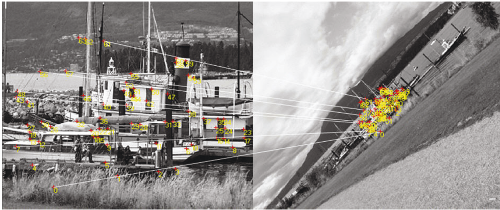
FIGURE 10: Matching result for image pair Boat (frames 0 and 9 of “Boat” sequence). The scale factor is 4.3, and the rotation angle is 45 degrees.
