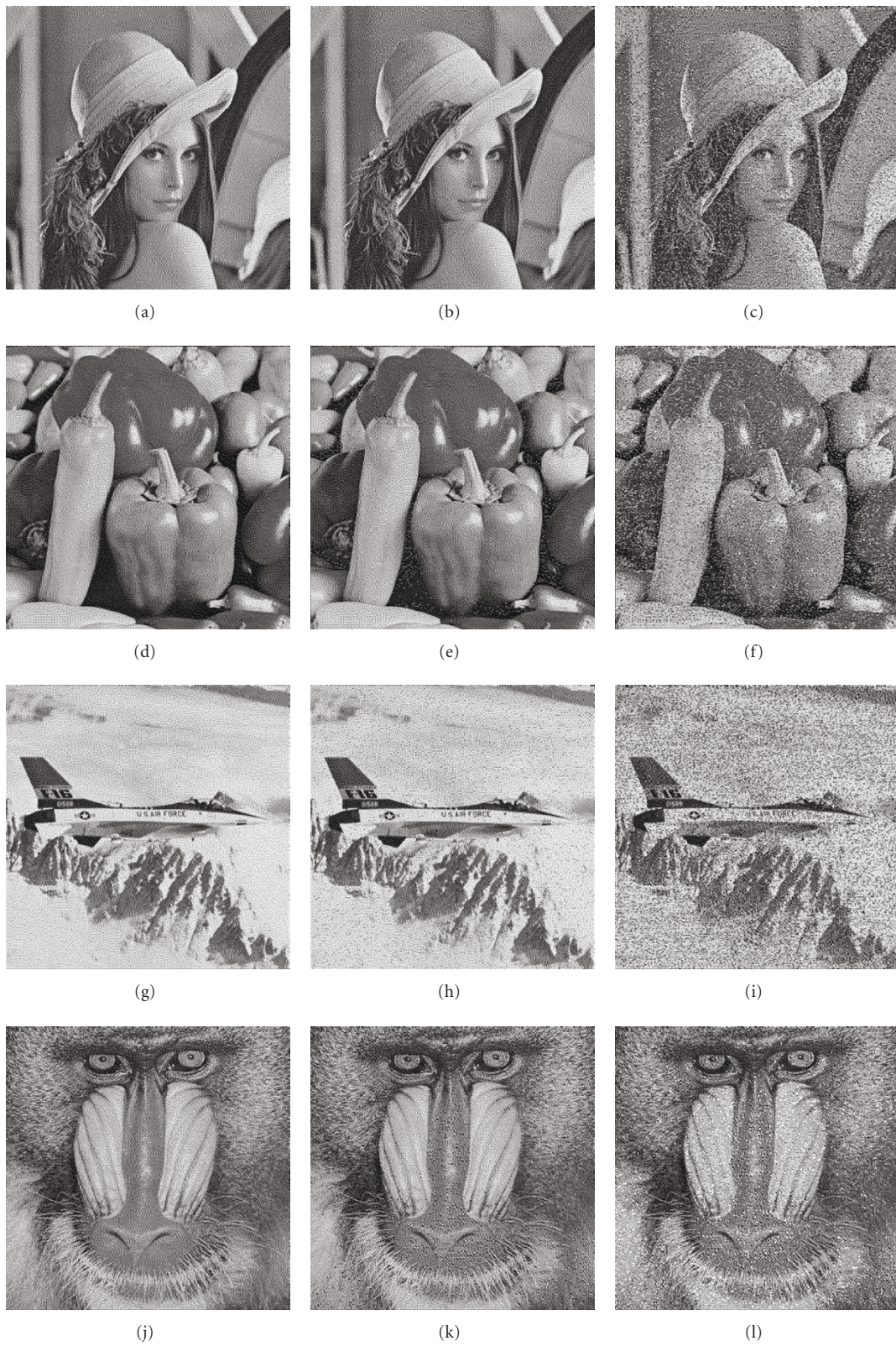
FIGURE 15: The stego images of data hiding using the proposed method: (a), (d), (g), and (j) the halftone image generated by error diffusion; (b) and (h) the stego images of embedding two pairs of templates; (e) and (k) the stego images of embedding three pairs of templates; (c), (f), (i), and (l) the stego image of hiding all pairs of templates.
