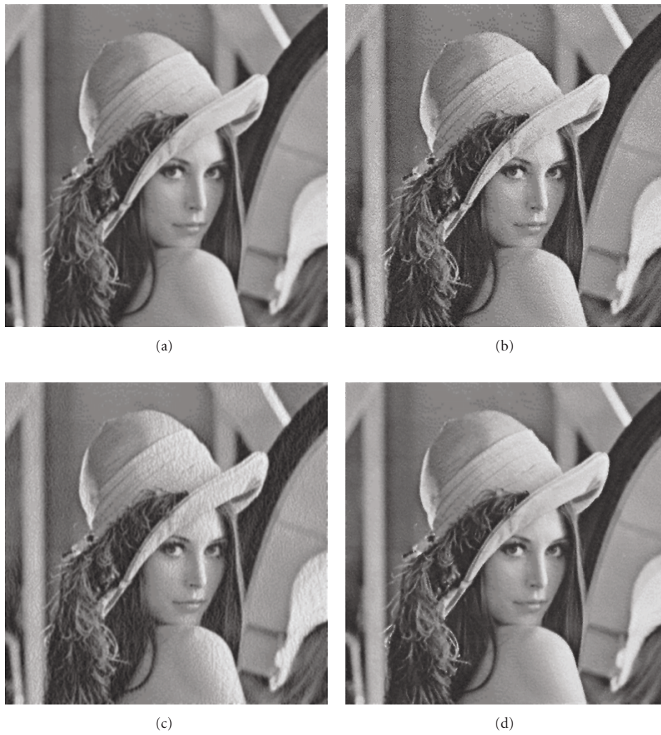
FIGURE 17: The inverse half-toning results using different methods: (a) the reconstructed image using Gaussian filtering; (b) the reconstructed image using LUT method; (c) the reconstructed image using ELUT method; (d) the reconstructed image using the proposed method.
