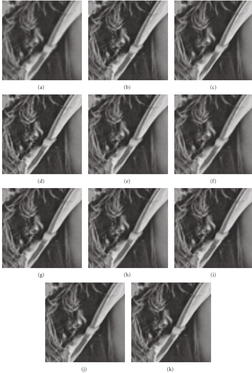
FIGURE 15: Portions of resolution enhanced “Lena” image (downsampled by averaging) by (a) bilinear; (b) bicubic; (c) edge-directed method ( M = 8 ) [12]; (d) ICBI [20]; (e) LMMSE-based method ( \zeta = 1, \xi = 1.5 ) [17]; (f) SAI ( \lambda = 0.5 ) [18]; (g) NN-based method [16]; the proposed method utilized (h) bilinear kernel and (i) bicubic kernel without edge enhancement; (j) bilinear kernel and (k) bicubic kernel with edge enhancement.
