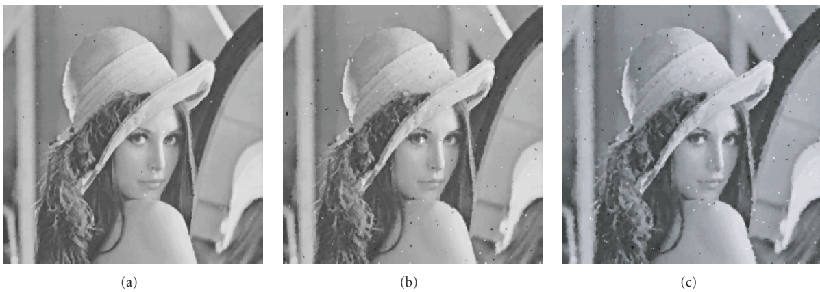
FIGURE 4: Using 3 \times 3 dichotomous WOS filter to restore (a) 5% impulse noise image; (b) 10% impulse noise image; (c) 15% impulse noise image.
