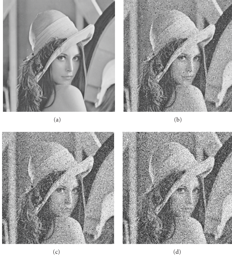
FIGURE 2: (a) Original “Lenna” image; (b) “Lenna” image corrupted by 5% impulse noise; (c) “Lenna” image corrupted by 10% impulse noise; (d) “Lenna” image corrupted by 15% impulse noise.
