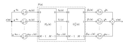
FIGURE 4: Polyphase representation of the analysis and the synthesis filters.
