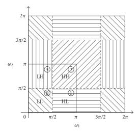
FIGURE 2: Four-band split of 2D spectrum.
