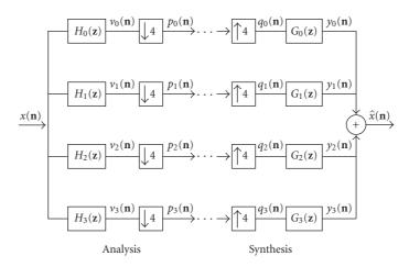
FIGURE 1: Two-dimensional four-channel filter bank.
