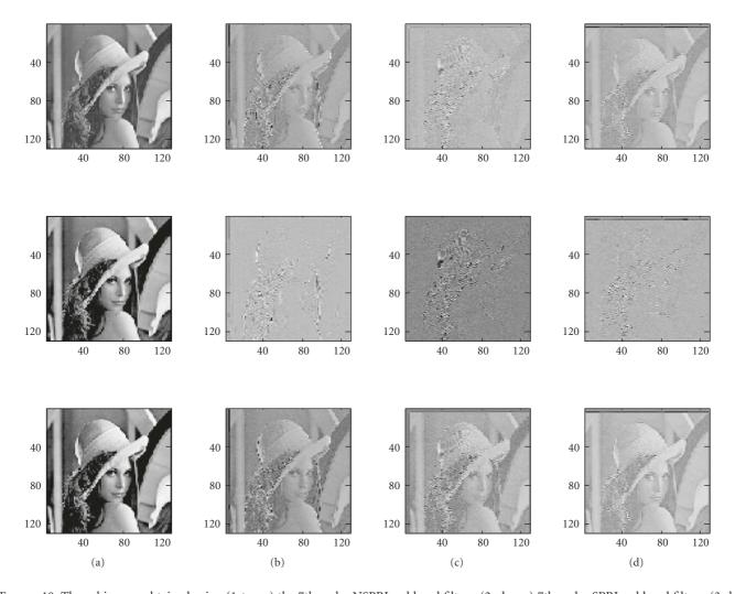
FIGURE 10: The subimages obtained using (1st row) the 7th-order NSPRL subband filters; (2nd row) 7th-order SPRL subband filters; (3rd row) 7th-order 3PLF subband filters. For  $(\omega_{s_1}, \omega_{s_2}) = (0.22\pi, 0.22\pi)$ . (a) LL subimages; (b) HL subimages; (c) HH subimages; (d) LH subimages.
