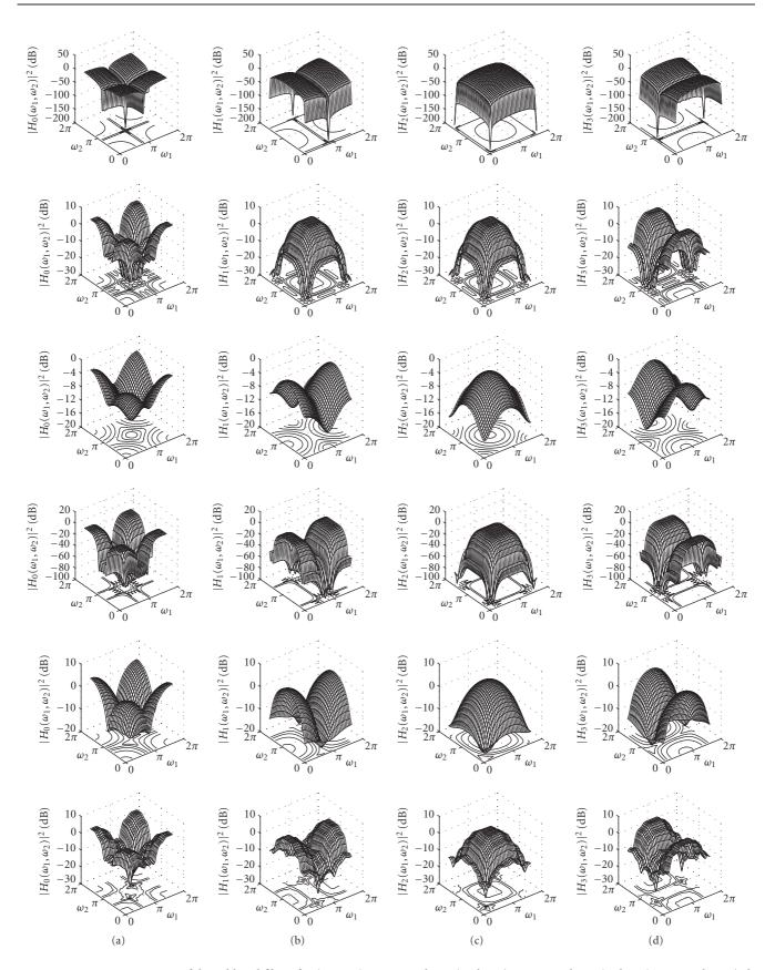
FIGURE 9: Frequency reponses of the subband filters for (1st row) NSPRL order 1; (2nd row) NSPRL order 7; (3rd row) SPRL order 1; (4th row) SPRL order 7; (5th row) 3PLF order 1; (6th row) 3PLF order 7. Cut-off frequencies for the HH filter are  $(\omega_{s_1}, \omega_{s_2}) = (0.22\pi, 0.22\pi)$ . (a) LL filters; (b) HL filters; (c) HH filters; (d) LH filters.
