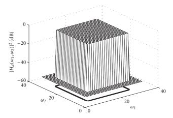
Figure 8: Frequency response of the desired HH filter;  $(\omega_{s_1}, \omega_{s_2}) = (0.22\pi, 0.22\pi)$ .
