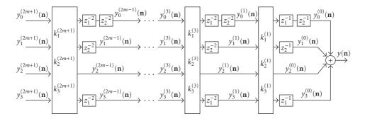
FIGURE 7: The synthesis section of the NSPRL filter bank.
