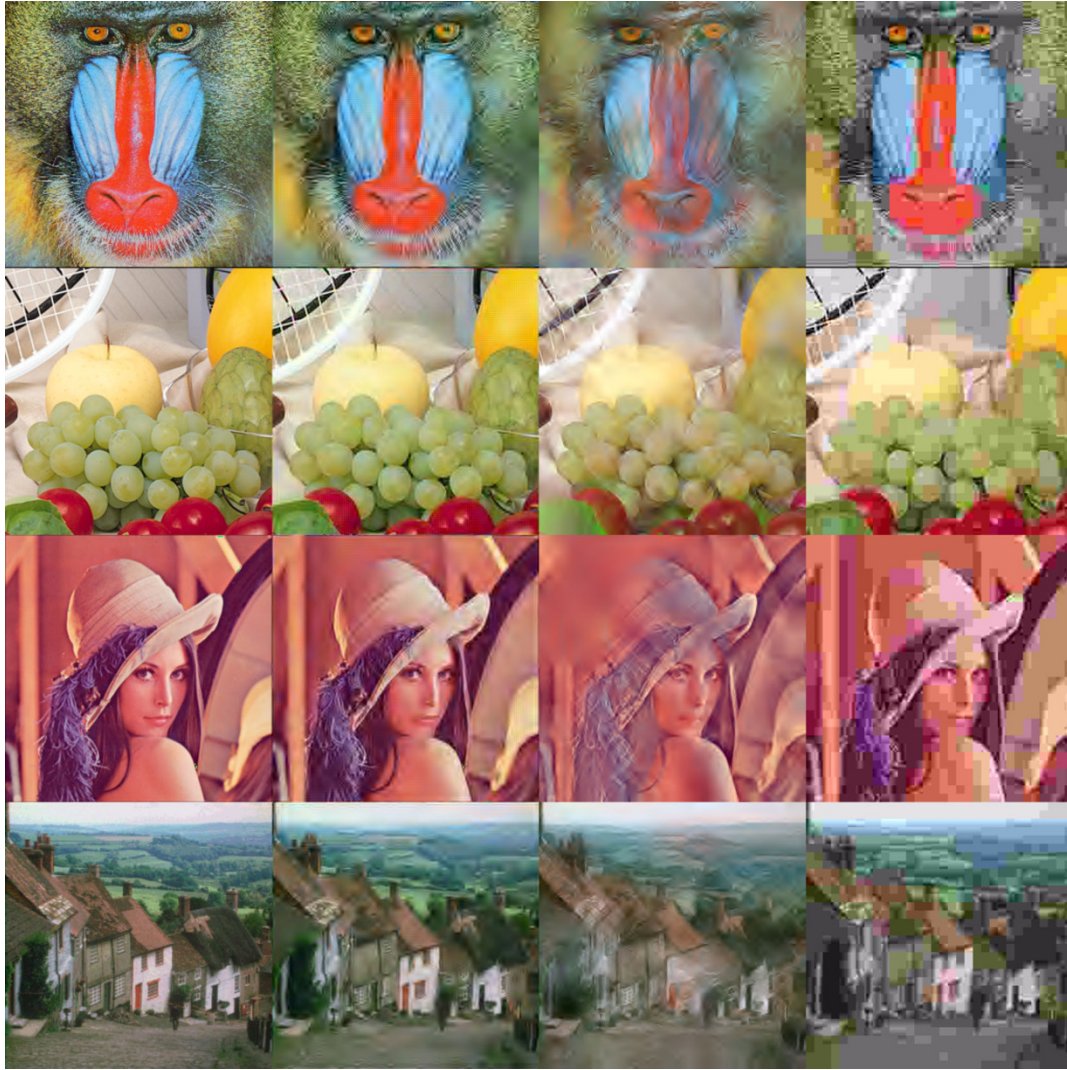
FIGURE 6: For each row from left to right: original color image (24 bits/pixel), compressed image using the proposed approach (0.30 bits/pixel), compressed image using SPIHT (0.30 bits/pixel), and compressed image using the JPEG method (0.30 bits/pixel). First row: “Baboon,” second row: “Biked,” third row: “Lena,” fourth row: “GoldHill.”
