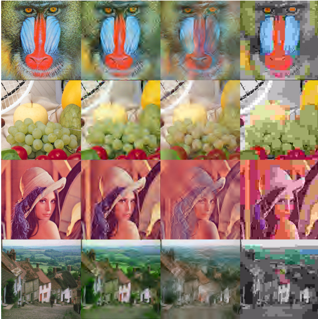
FIGURE 5: For each row from left to right: original color image (24 bits/pixel), compressed image using the proposed approach (0.15 bits/pixel), compressed image using SPIHT (0.15 bits/pixel), and compressed image using the JPEG method (0.25 bits/pixel (maximum compression rate allowed by the JPEG coder)). First row: “Baboon,” second row: “Biked,” third row: “Lena,” fourth row: “GoldHill.”
