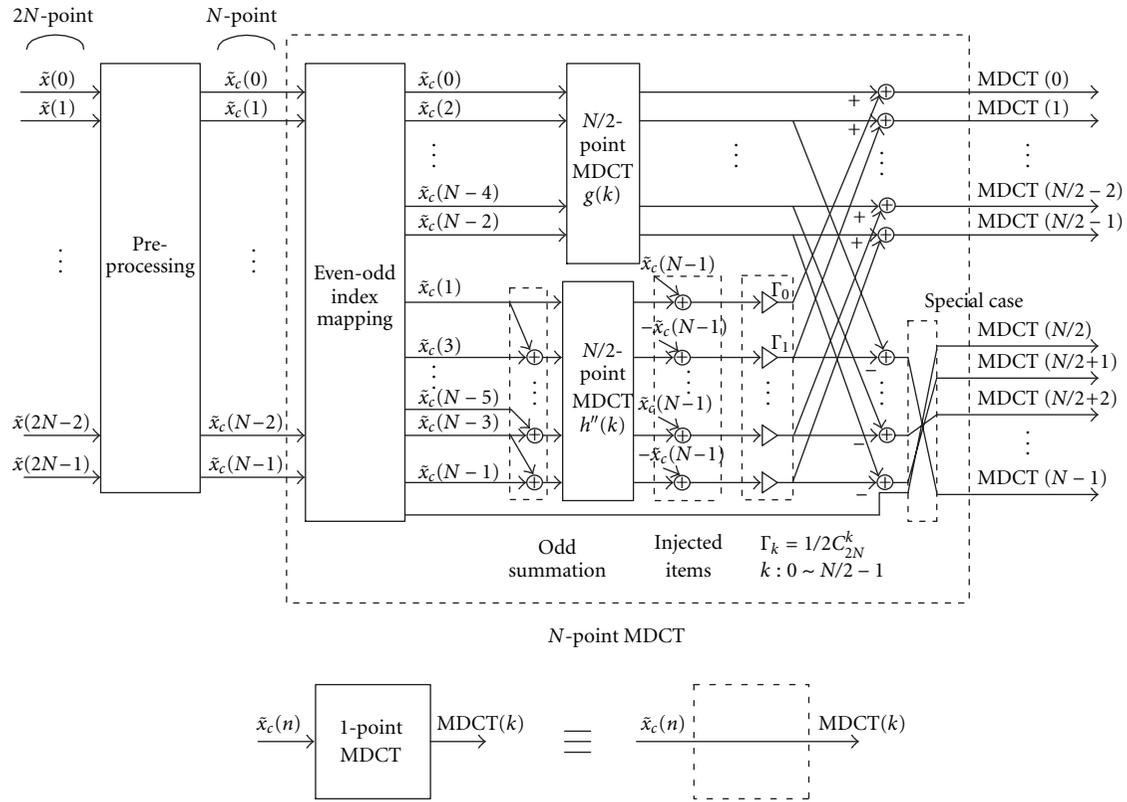
FIGURE 7:  $N$ -point MDCT( $k$ ) butterfly structure, where 1-point MDCT is the minimum-sized processing block of the FFT module.
