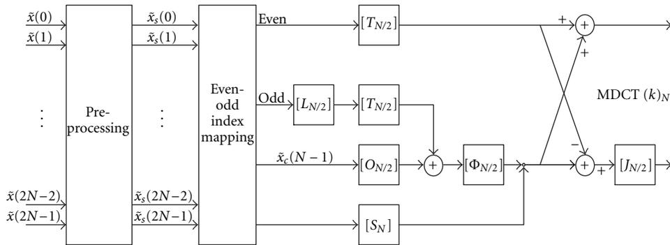
FIGURE 10: Block diagram of the MDCT in matrix form for the FFT operation.
