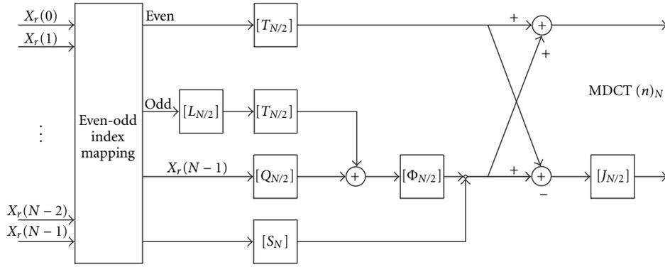
FIGURE 5: Block diagram of the MDCT operation in matrix form.
