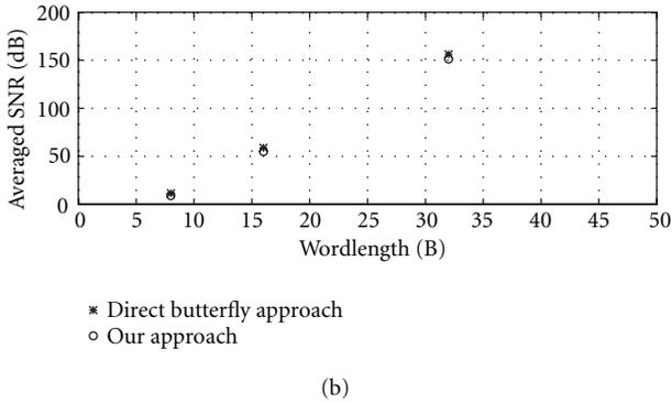
FIGURE 12: Averaged SNR versus wordlength for the 512-point ( $2N$  value) (a) IFFT. (b) FFT.
