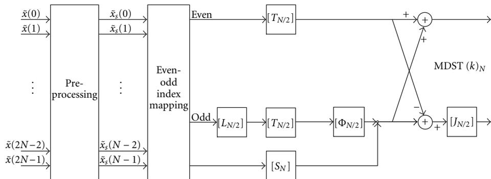
FIGURE 11: Block diagram of the MDST in matrix form for the FFT operation.
