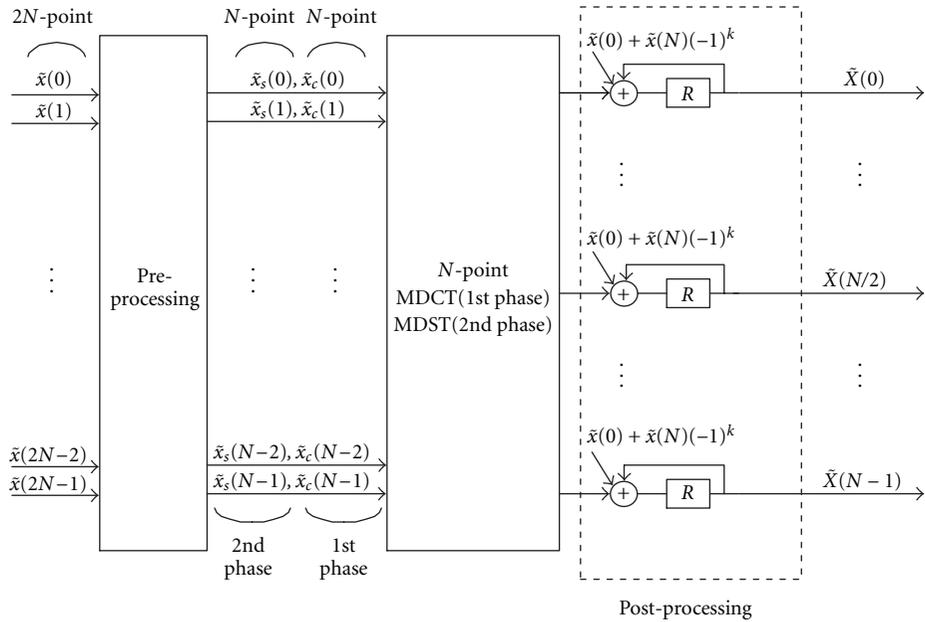
FIGURE 9: The proposed FFT architecture.
