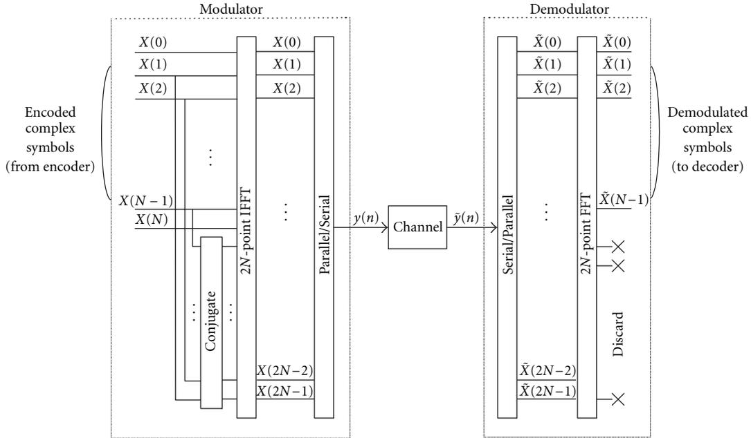
FIGURE 1: The IFFT/FFT block diagram in the DMT system.
