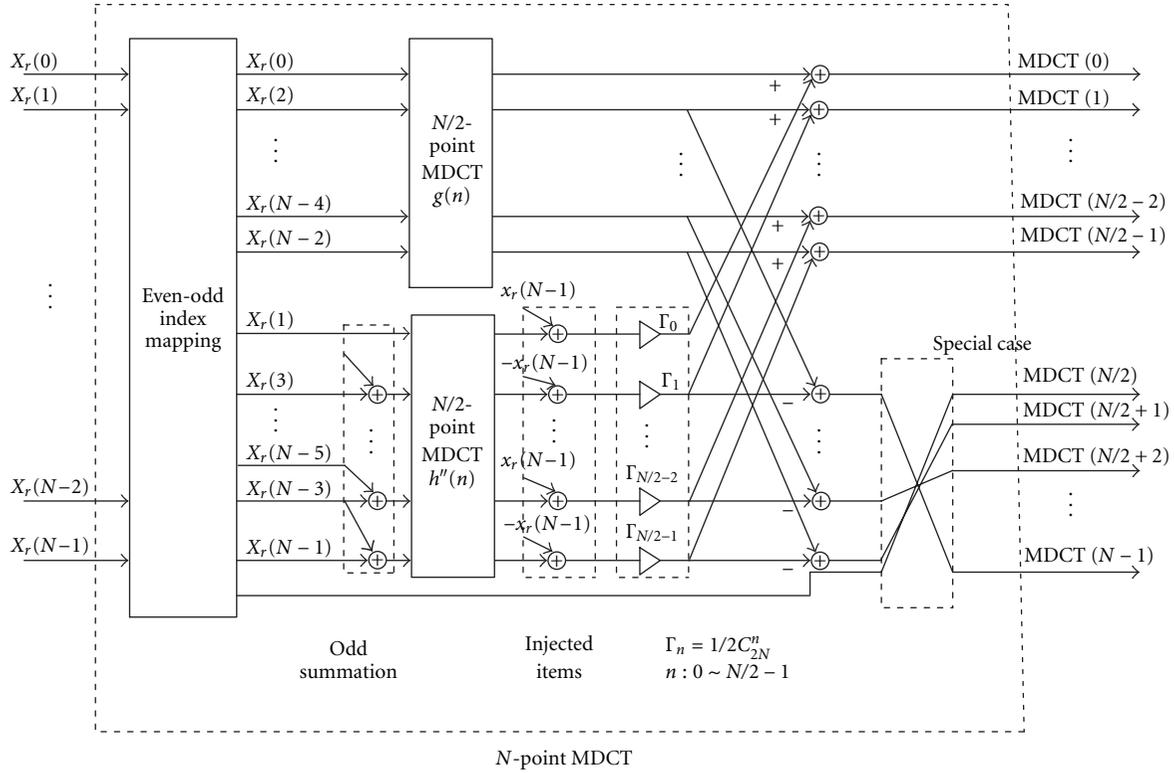
FIGURE 2:  $N$ -point  $\text{MDCT}(n)$  butterfly structure, where 1-point MDCT is the minimum-sized processing block.
