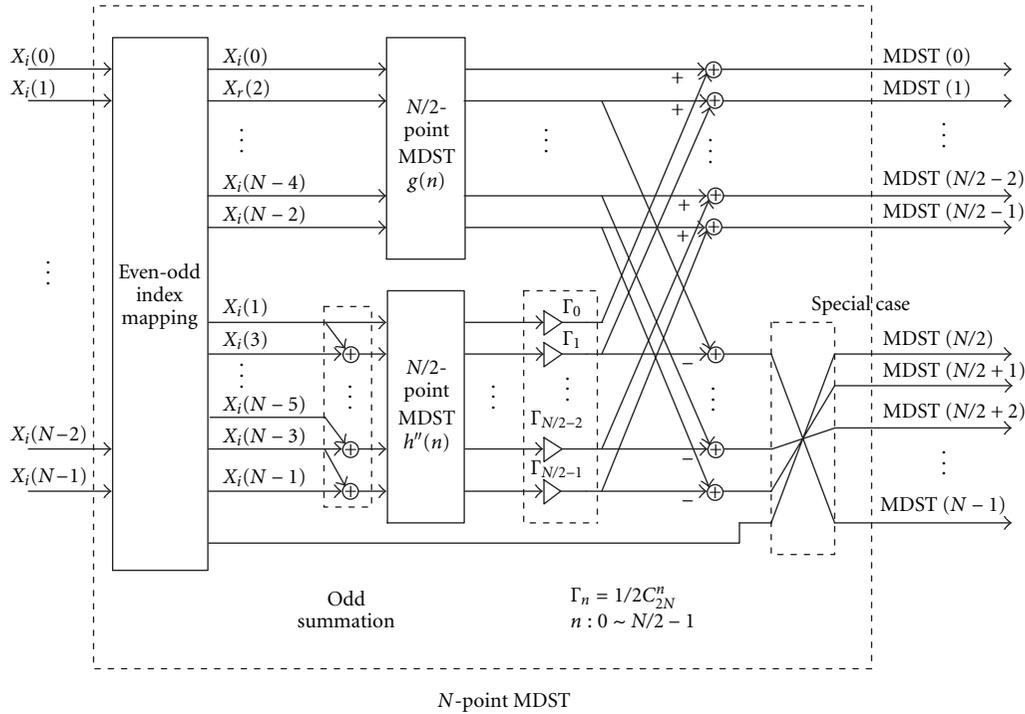
FIGURE 3:  $N$ -point MDST( $n$ ) butterfly structure, where 2-point MDST is the minimum-sized processing block.
