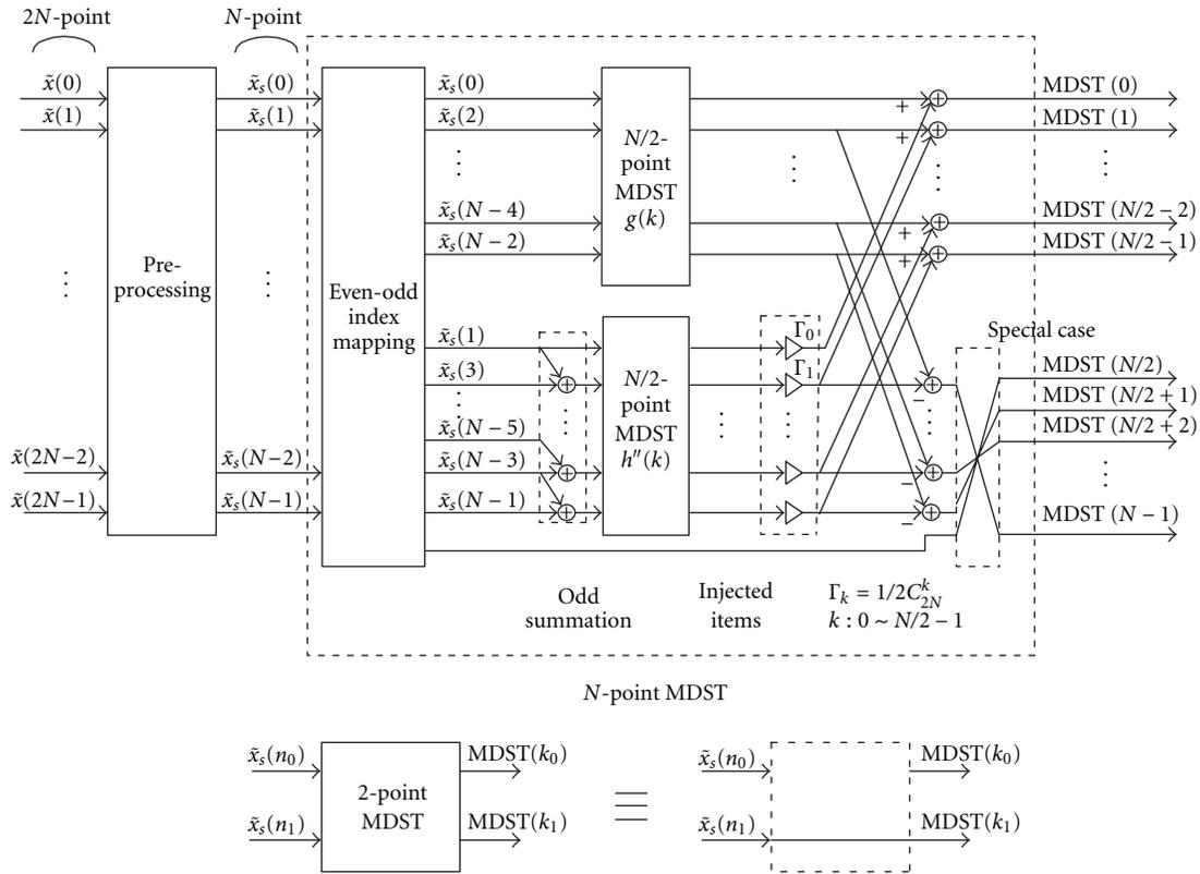
FIGURE 8:  $N$ -point MDST( $k$ ) butterfly structure, where the 2-point MDST is the minimum-sized processing block of the FFT module.
