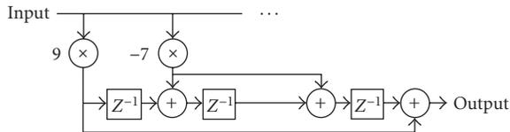
FIGURE 1: Modified transversal filter architecture implementing coefficient set  $\{9, -7, -7, 9\}$ . Coefficient multipliers are shared for duplicated coefficients in the coefficient set.
