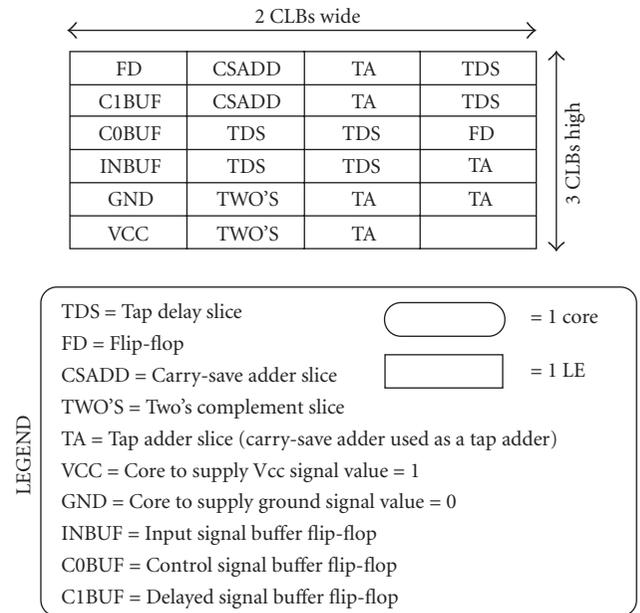
FIGURE 8: The result of folding the physical serial map to fit a bounding box three CLBs high and two CLBs wide.
