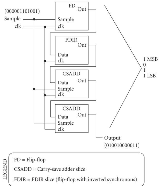
FIGURE 3: Serial-by-parallel constant coefficient multiplier for coefficient eleven, constructed from bit-serial component library. A control signal is not shown to simplify the diagram.
