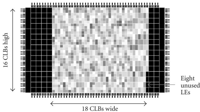
FIGURE 11: Visualization of bit-serial component library subcores as they are placed in a bit-serial FIR filter core with 95 taps and a PSR of 49.9 dB. The device shown is the VirtexDS simulation of the Xilinx Virtex XCV50 part, the smallest Virtex device.
