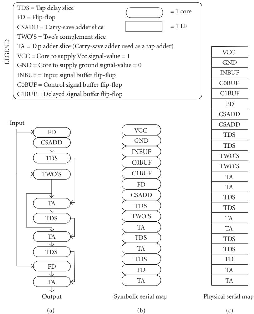
FIGURE 5: (a) Transposed FIR filter architecture rearranged into a column of cores for coefficients  $\{1, -1, -1, 3\}$ . (b) Symbolic serial map generated by the serial mapper for coefficient set  $\{1, -1, -1, 3\}$ . The symbolic serial map corresponds to the transposed FIR filter architecture rearranged in (a). (c) Physical serial map generated by the serial mapper for coefficient set  $\{1, -1, -1, 3\}$ , corresponding to the symbolic serial map in (b).
