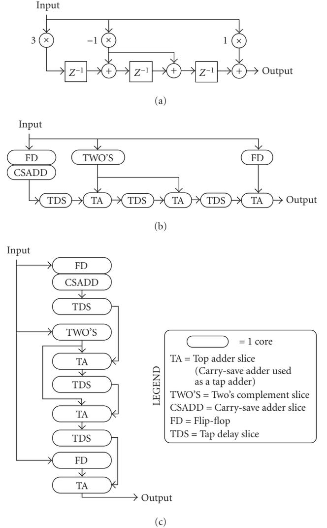
FIGURE 4: (a) Transposed FIR filter architecture for coefficient set  $\{1, -1, -1, 3\}$ . (b) Cores substituted into the transposed FIR filter architecture to create constant coefficient serial-by-parallel multipliers, tap adders, and tap delays. (c) Transposed FIR filter architecture rearranged into a column of cores.
