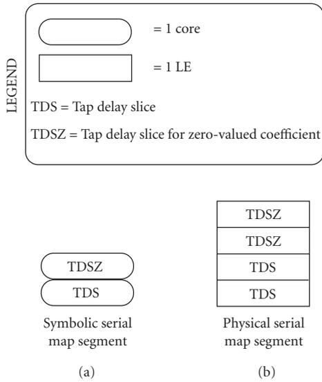
FIGURE 6: Mapping a zero coefficient. (a) Symbolic serial map segment for a zero-valued coefficient. (b) Corresponding physical serial map segment of a zero-valued coefficient.
