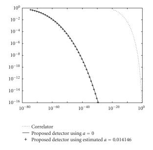
FIGURE 5: ROC curves of the normalized correlator, the proposed detector by using the known parameter a, and the proposed detector after estimating the parameter a, a = 0.
