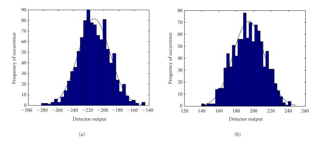
FIGURE 4: Empirical detector output distribution: (a) erroneous key and (b) correct key.
