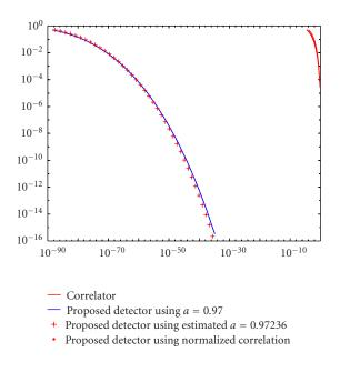
FIGURE 7: ROC curves of correlator, the normalized correlator, the proposed detector by using the known parameter a, and the proposed detector after estimating the parameter a, a = 0.97.
