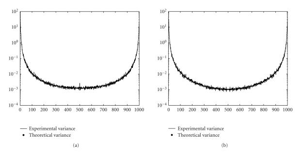
FIGURE 2: Theoretical and experimental variances of (a) real and (b) imaginary parts of each discrete Fourier coefficient of 100 signals of length 1000, having a = 0.99.
