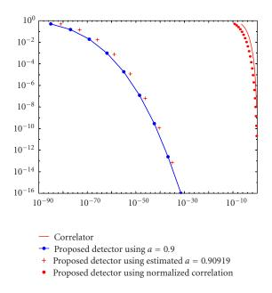
FIGURE 6: ROC curves of correlator, the normalized correlator, the proposed detector by using the known parameter a, and the proposed detector after estimating the parameter a, a = 0.9.
