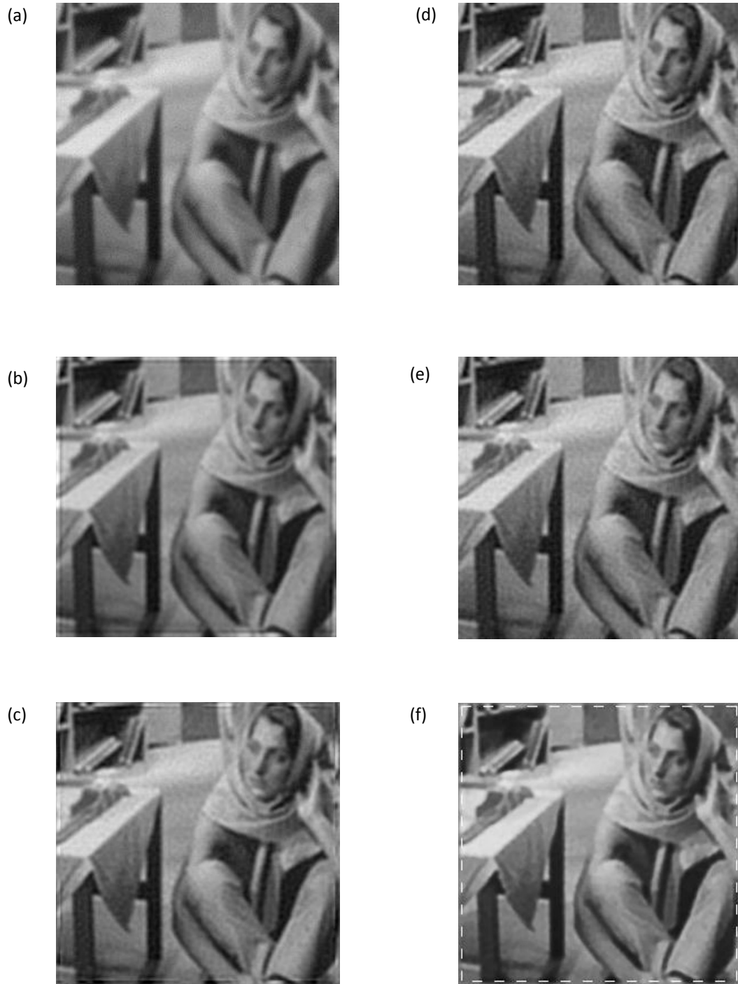
Figure 10 Restoration results from the Barbara degraded image by Gaussian blur 7 \times 7 and BSNR = 20 dB. (a). For the HyBR method, the restored images with BCs (b) zero: \sigma_e = 15.25 , (c) periodic: \sigma_e = 13.81 , (d) reflexive: \sigma_e = 12.99 and (e) anti-reflexive: \sigma_e = 12.98 . The MLP restored image (f) performs considerably better with \sigma_e = 12.47 in the original image size.
