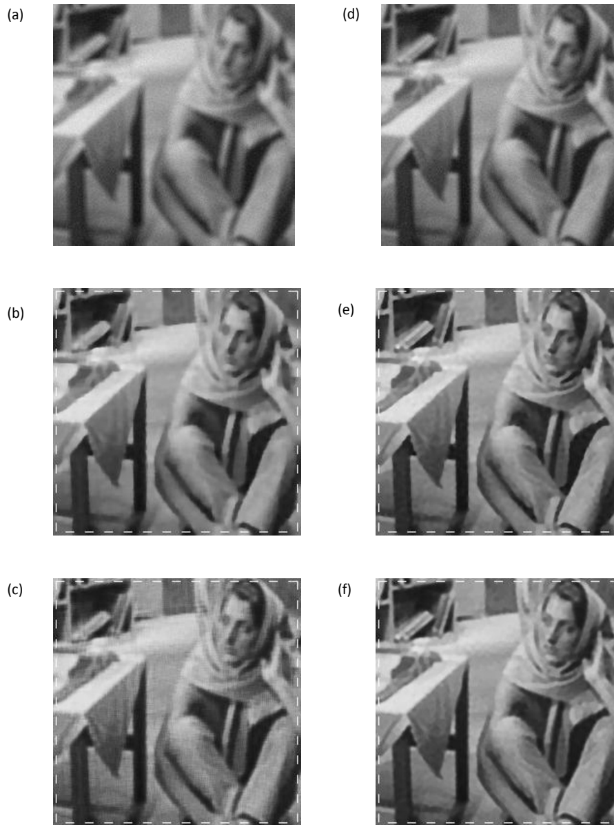
Figure 11 Restoration results from the Barbara degraded image by Uniform (a) and Gaussian (d) blurs 7 \times 7 and BSNR = 20 dB. For the Extrapolation method, the output images reach restoration errors of (b) \sigma_e = 13.23 and (e) \sigma_e = 12.49 , respectively, while in the MLP we compute values of (c) \sigma_e = 13.53 and (f) \sigma_e = 12.33 .
