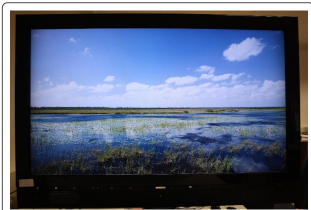
Figure 3 The captured image. This is an example image of the TV screen captured by the camera. TV screen boundary has at least two edges (inner and outer) which need to be detected by the algorithm. Algorithm should extract only the part of the image which represents the TV screen content—that is the part inside the inner boundary.
