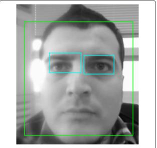
Figure 1 Face with eyes sockets detected by OpenCV AdaBoost classifier.
