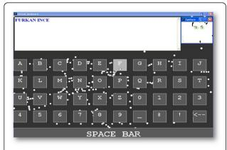
**Figure 13 Dwell-time-based virtual keyboard employed in 2D gaze estimation and cursor control experiment.** White circles are the saccades showing the gaze projectory path.
