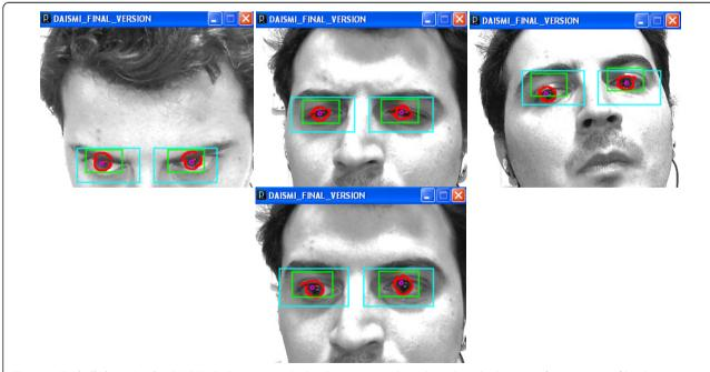
**Figure 4 Eyeball detection by DAISMI.** Red points are the border vertices and purple circle is the location of mass-center of border vertices in terms of low-intensities.
