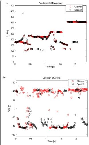
Figure 3 The estimates of (a) the fundamental frequency using maximum-likelihood estimator at the output of the beamformer, (b) the DOA using a delay-sum beamformer.
