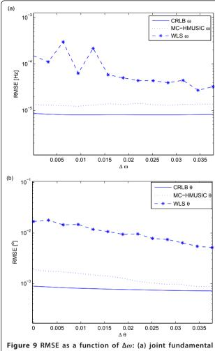
Figure 9 RMSE as a function of  $\Delta\omega$ : (a) joint fundamental frequency estimates; (b) joint DOA estimates.
