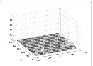
Figure 4 Example of cost functions for two synthetic sources having three harmonic each, N=64 and M=8. The true fundamental frequency of  $\omega_1=252.123$  and  $\omega_2=300.321$  having DOA  $\theta_1=-43.23^\circ$  and  $\theta_2=70^\circ$ , respectively.
