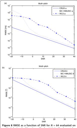
Figure 8 RMSE as a function of SNR for N = 64 evaluated or multi-pitch signal with unit amplitudes: (a) joint fundamental frequency estimates; (b) joint DOA estimates.
