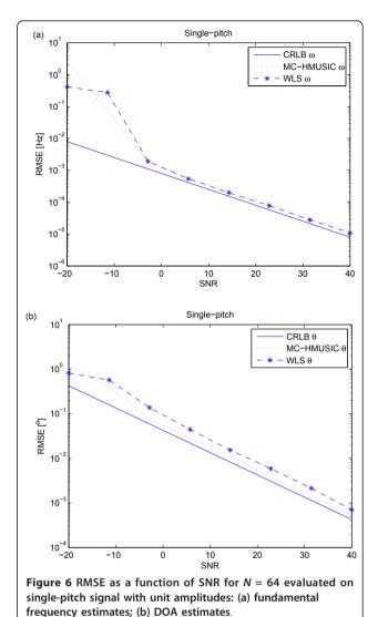
on single-pitch signal with unit amplitude: (a) fundamental frequency estimates; (b) DOA estimates.
