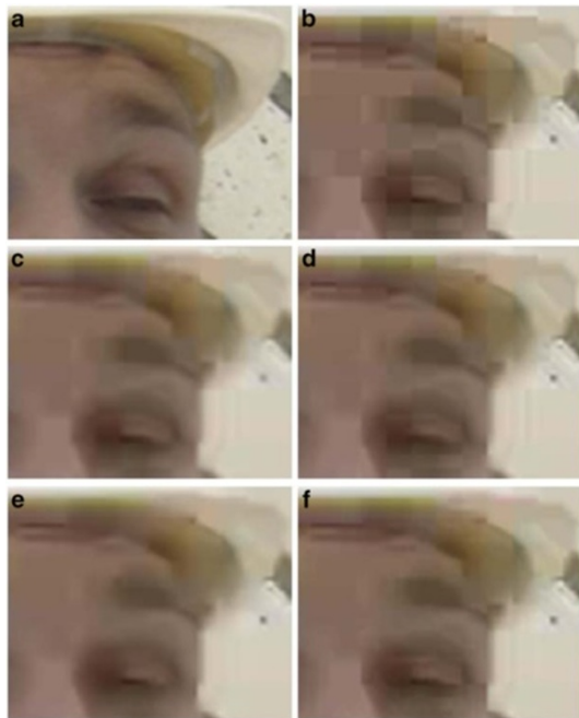
Figure 19 Details of the blue region in Foreman (CIF, Frame #1, target bit-rate: 105 kbps). (a) The original frame, (b) non-filtered frame, (c) filtered by Tai's [18] 4 \times 4 filter, (d) filtered by Chen's [19] filter, (e) filtered by H.264/AVC loop filter [20], and (f) filtered by the proposed algorithm.
