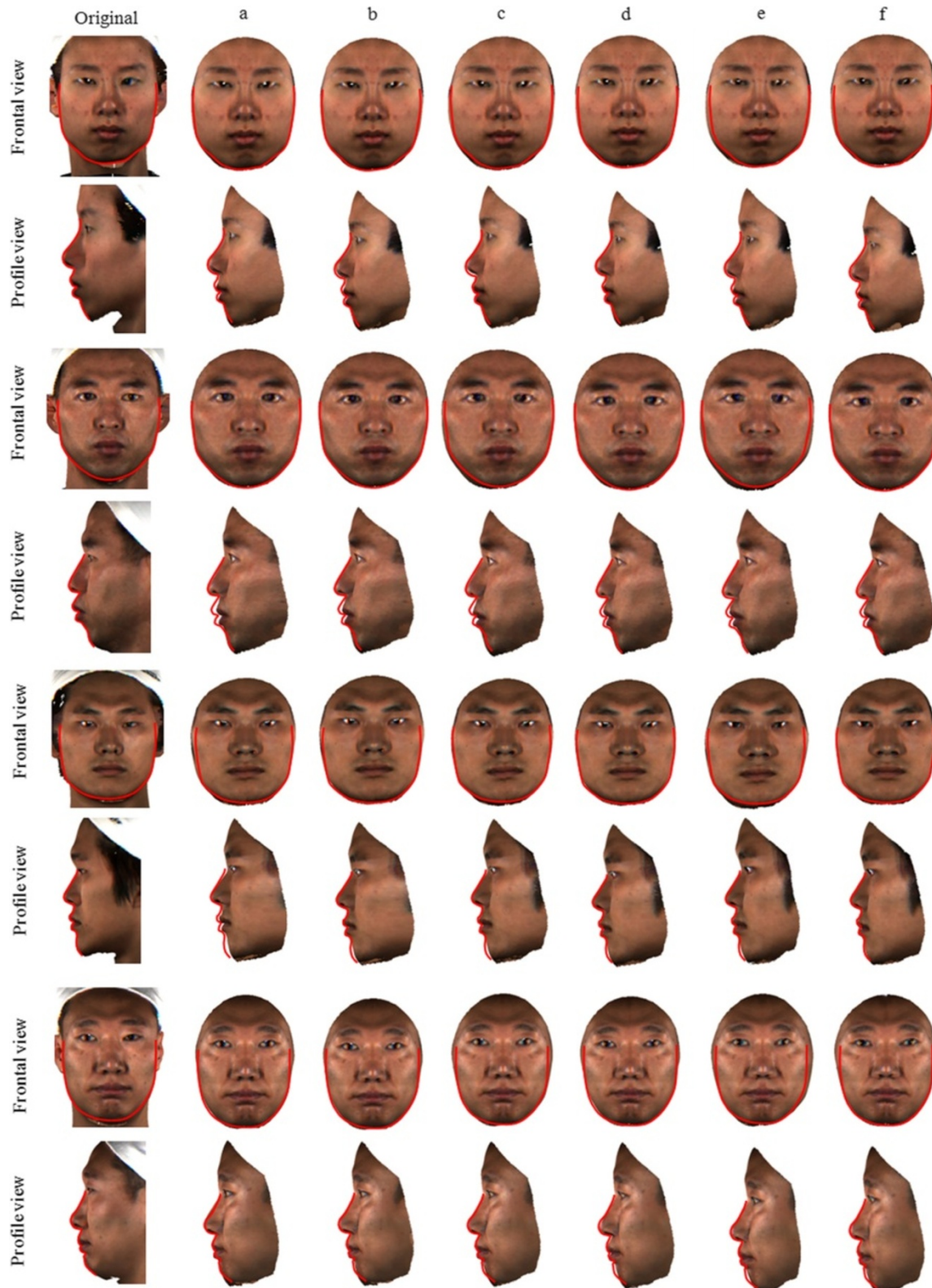
Figure 17 Examples of faces reconstructed using Test data 1 (a, b: previous method and proposed method at 15°; c, d: previous method and proposed method at 30°; e, f: previous method and proposed method at 45°; red solid lines represent the accurate frontal and profile shapes of the ground-truth face)
