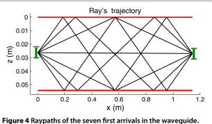
Red horizontal lines represent the air-water interface and the waveguide bottom. Green vertical lines represent the source and receiver arrays. The raypaths are plotted between the centers of the source and receiver arrays.
