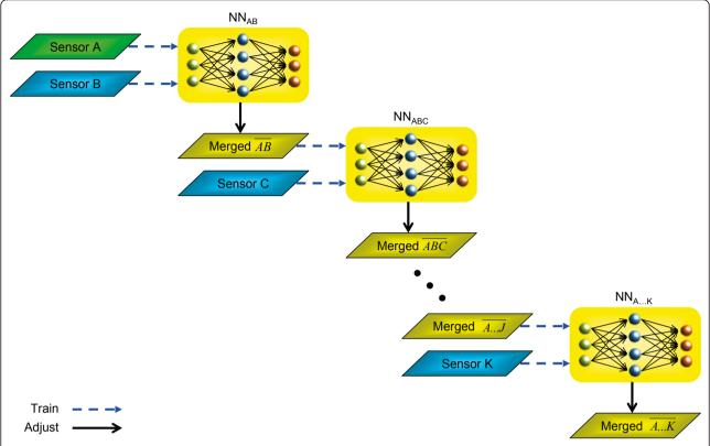
**Figure 1 Schematic representation of SNN for merging multi-sensor datasets**. The dashed arrows represent the training phase; the continuous arrows represent the application of the adjustments computed by the neural network.
