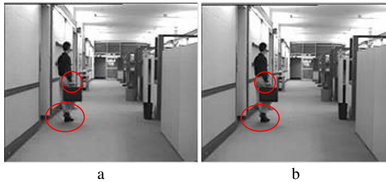
Figure 8 Reconstructed frame #17 in Hall monitor with (a) DISCOVER scheme and (b) the proposed one.
