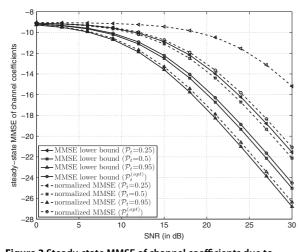
Figure 3 Steady-state MMSE of channel coefficients due to Kalman channel tracking.
