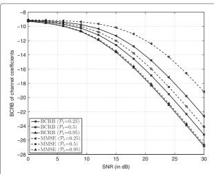
Figure 1 Bayesian CRB and MMSE of channel coefficients.
