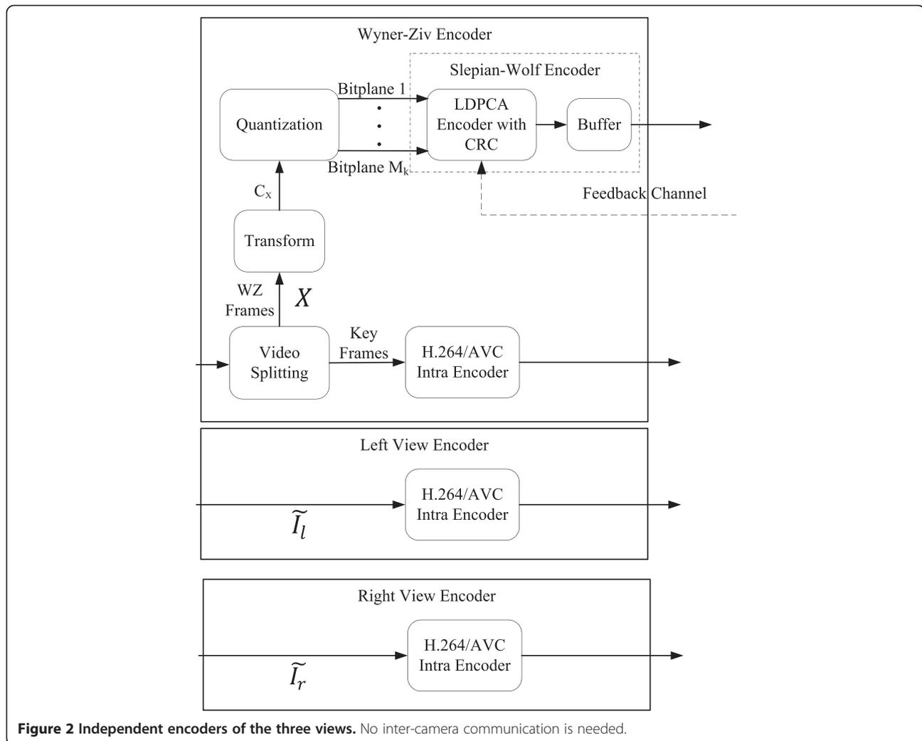
**Figure 2** Independent encoders of the three views. No inter-camera communication is needed.
