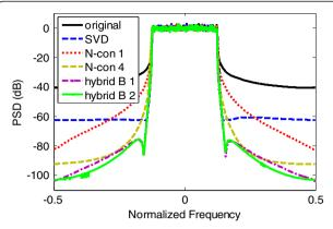
Figure 7 PSD of SVD precoding, *N*-continuous symbol mapping, and their combination with CP.
