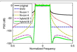
**Figure 6** PSD of SVD precoding, *N*-continuous symbol mapping, and their combination without CP.
