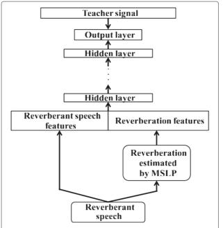
**Fig. 4** DNN structure using reverberation estimated by MSLP for environment identification and one-step environment-dependent DAE. The teacher signal is the label of environment for environment identification and MFCC of clean speech for the one-step environment-dependent DAE, respectively
