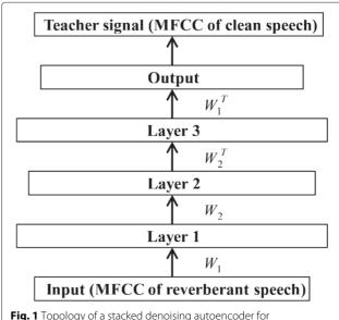
**Fig. 1** Topology of a stacked denoising autoencoder for cepstral-domain dereverberation
