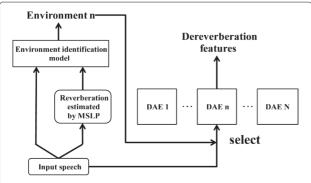
**Fig. 5** Flowchat of environment-dependent DAE and automatic environment identification
