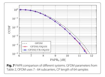
application of offset-QAM modulation, which can reduce PAPR. Furthermore, the figure shows equal PAPR for both GFDM/OQAM and GFDM/CR-OQAM.
