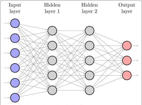
**Fig. 2** Feed-forward network with an input layer where the TF features are inserted, two hidden layer consisting of several hidden nodes, and an output layer for classification into three categories
