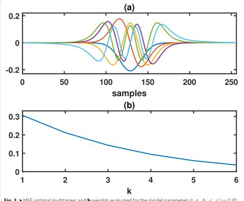
**Fig. 3 a** MSE optimal multitapers and **b** weights evaluated for the model parameters (L,  $a_q$ ,  $b_q$ ,  $c_q$ ,  $c_r$ ) = (120, 500, 0.20, 800, 15,000)
