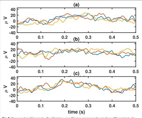
**Fig. 9** Three random EEG signals, after 70 Hz low-pass filtering, corresponding to three different trials of a memory task, from each category: **a** "Faces," **b** "Objects," and **c** "Landmarks"
